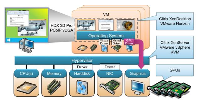
Citrix XenServer 6.x and VMware vSphere 5.1 or higher support the pass-through or direct attached GPU for Virtual Desktops.
