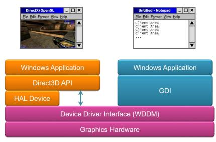
If an adequate graphics card is available, Direct3D can use it for hardware acceleration of the entire 3D rendering pipeline or part of it. The advanced graphics capabilities of the underlying 3D graphics hardware are exposed through Direct3D. Combining such capabilities with the other DirectX technologies allows for advanced multimedia scenarios.
