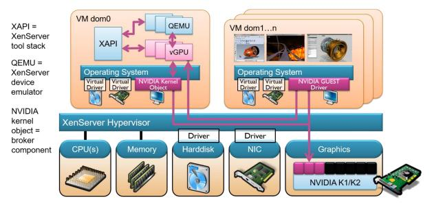
NVIDIA GRID technology offers the ability to offload graphics processing from the CPU to the GPU in 3D graphics for virtual desktop environments, allowing the data center manager to deliver true PC graphics-rich experiences to more users for the first time.
