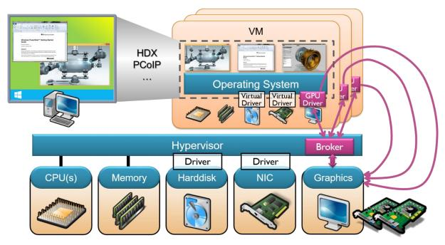
In the case of NVIDIA GRID each VM is configured with a vGPU profile with a configurable static vRAM size and the VM will share GPU processing power. Citrix XenServer and VMware ESXi/vSphere are the virtualization hypervisors in the market that supports NVIDIA GRID vGPU.
