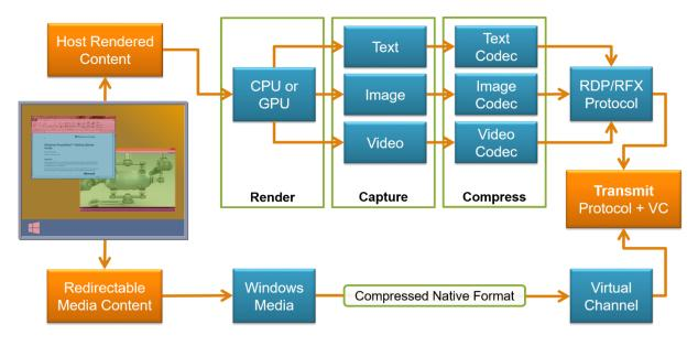
Typically, the entire screen goes through the RemoteFX render-capture-compress pipeline at 30 frames per second, except for redirected multimedia, such as WMV streams. Redirected media content is directly transmitted to the client in its compressed native format using an RDP virtual channel.
