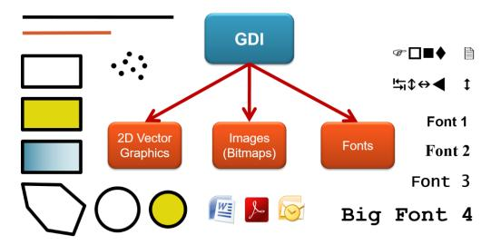
It is important to note that GDI was designed in such a way that it can be hardware accelerated in a graphics card. Every modern PC graphics card supports the full GDI function set in hardware. During the Windows initialization phase, GDI hardware acceleration is registered in the system, significantly reducing CPU load generated by graphics output during system runtime.
