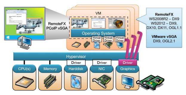
The advantage of GPU sharing is its superior scalability, delivering 10s of VMs or sessions per physical GPU which allow knowledge workers and task workers hardware-accelerated access to Line-of-Business applications and Windows desktops.
