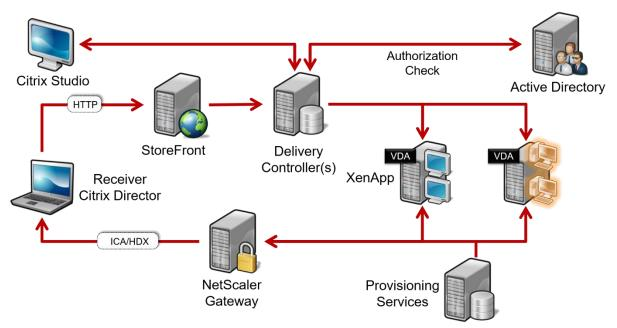
A XenDesktop agent is required in the guest VM or Blade PC. The agent enables direct connections between the endpoint and the user's virtual desktop. On the endpoint the Citrix Receiver or Receiver for HTML5 can be used to provide simple access from any device, anywhere, to virtual desktops and applications. The Citrix Receiver provides the most comprehensive experience, while the Receiver for HTML5 has less endpoint requirements as well as capabilities.
